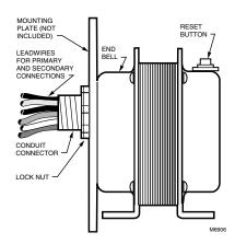
Fig. 2. Conduit/panel mounting (plate not included).
